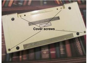
With the rear of the Electron facing towards you, remove the cover, remove the three screws holding the power circuitry on the left and the four screws
