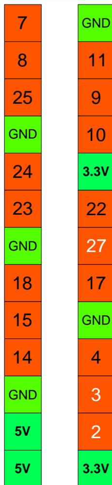
Fig.1 GPIO pinout
