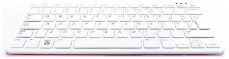
BBC Microcomputer Model A. 8 colours, 16K RAM, 2MHz, 3700g. Raspberry Pi 400. 16M colours, 3968MB RAM, 1.8GHz, 386g.
