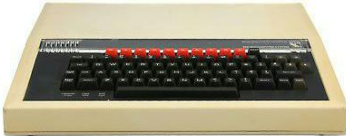
BBC Microcomputer Model A. 8 colours, 16K RAM, 2MHz, 3700g. Raspberry Pi 400. 16M colours, 3968MB RAM, 1.8GHz, 386g.
